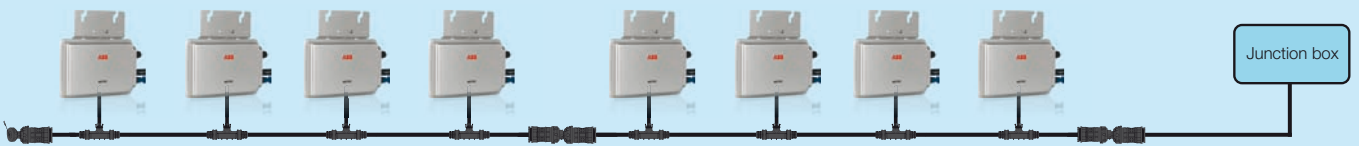
Small plant, more than four MICRO AC TRUNK BUS and two mounting accessories kit*
